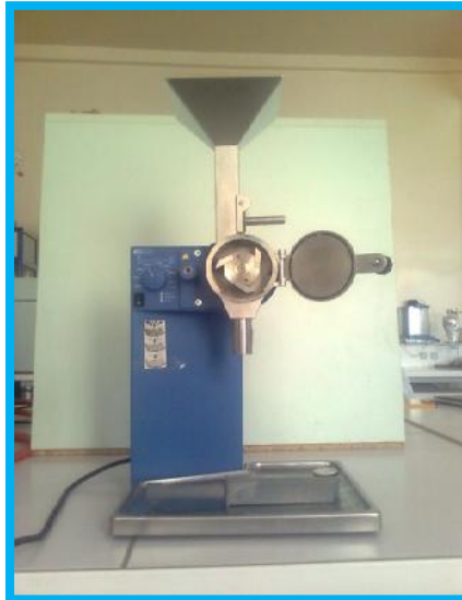
Figure 22. Moulin de laboratoire (MF 10 BASIC).
