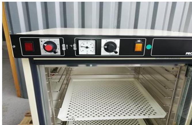
**Figure III-26 Etuve de séchage**
