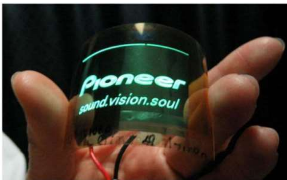
Figure 24: OLED, the organic light-emitting diode. (Okahisa et al., 2009)
